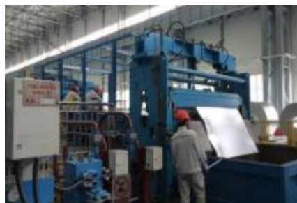
Surface Quality Inspection of Hot Rolled Coils
