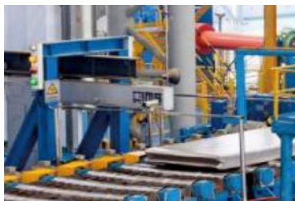
Rough roll mill exit IMS crown tester
