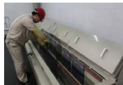
Anodized surface inspection of hot rolled plates
